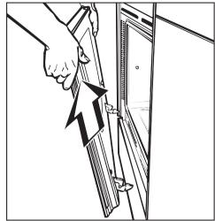
■ Lift up the door until the hinges disengage. Remove door.
